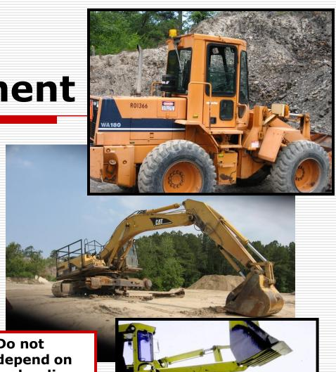
Do not depend on hydraulics for support, block and chock it!!
