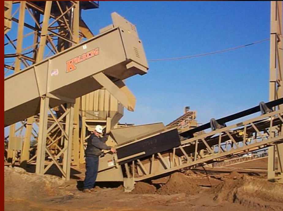
Miner ensuring guards are in place prior to starting equipment.
