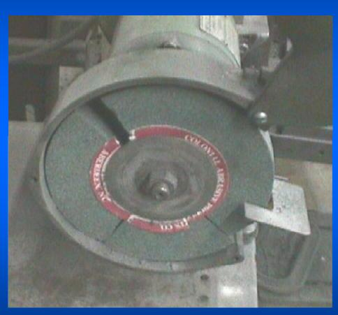
Spindle guard removed for better viewing
