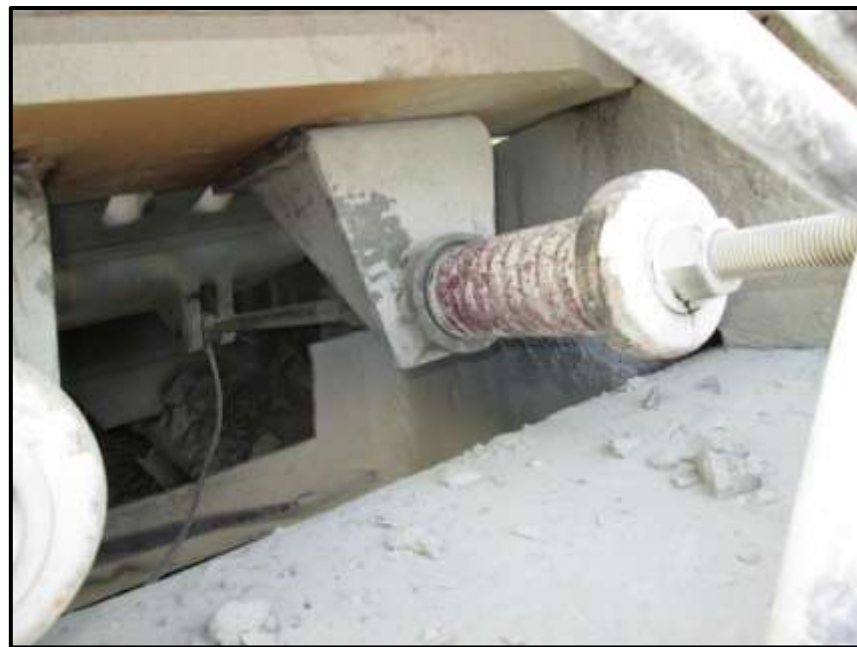
Tension rod assembly involved in this accident.
