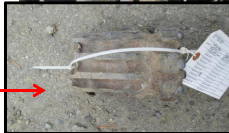
Broken drill bit that struck the miner
