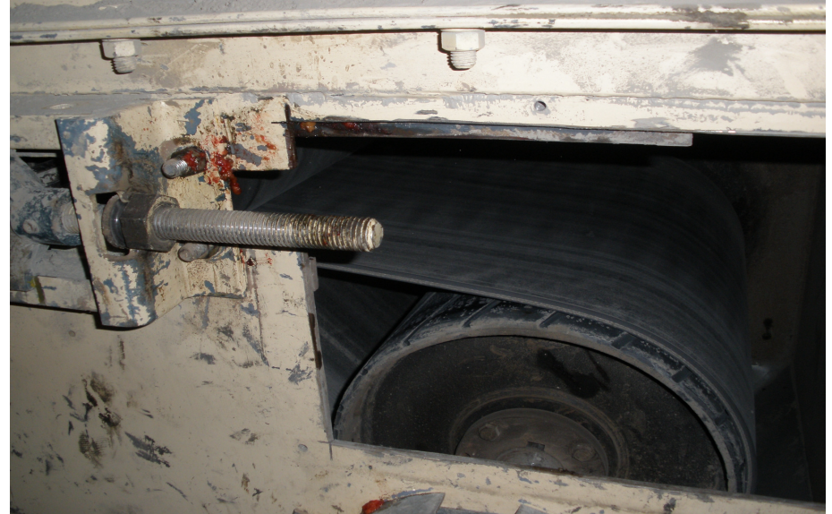
Access cover removed, showing area where miner was injured.
