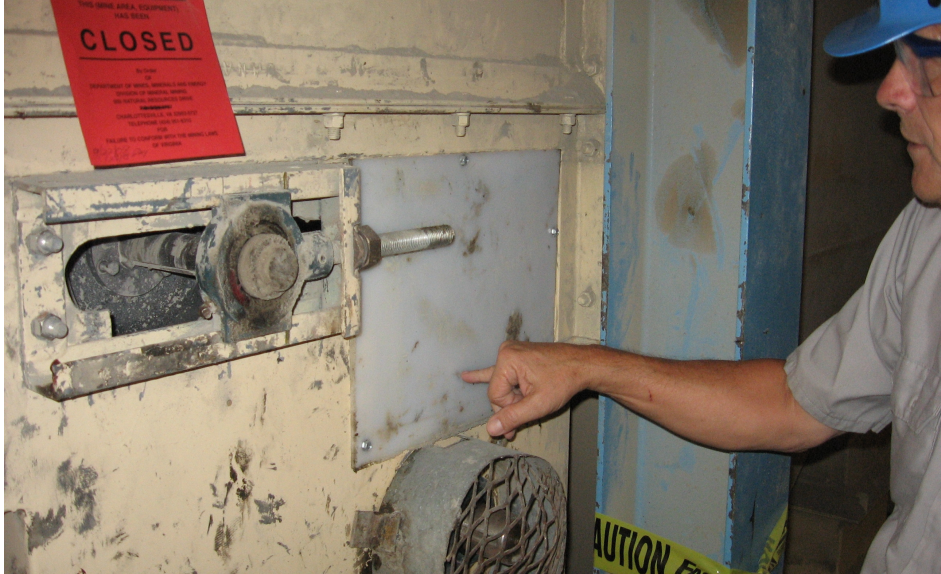
DMM inspector points to access cover that was removed.
