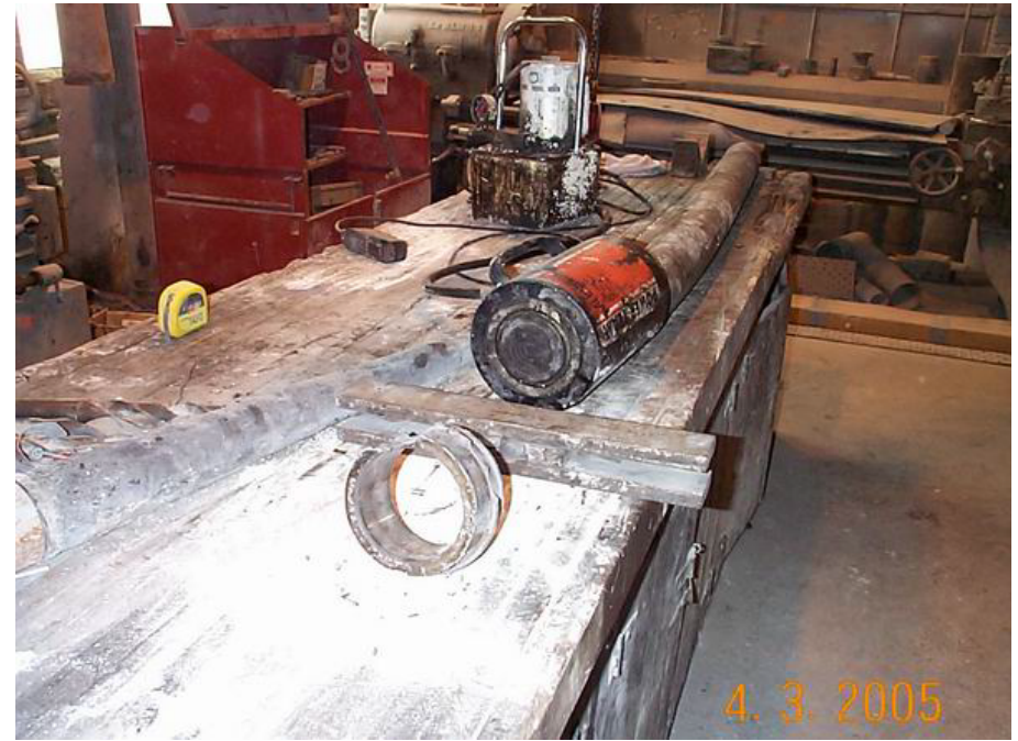
The metal ring and metal bar in the foreground of this photo were positioned between the port-a-power jack and the ram assembly.
