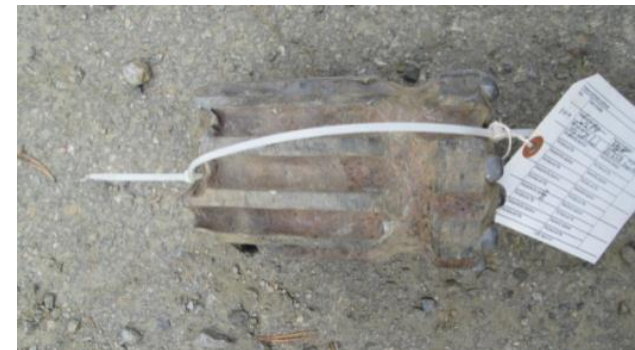
Portion of bit that struck the miner
