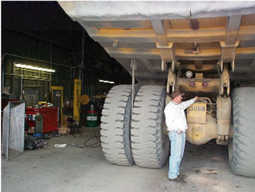
Lube points on the Komatsu haul truck with the Graco chassis pump out of sight in the background.
