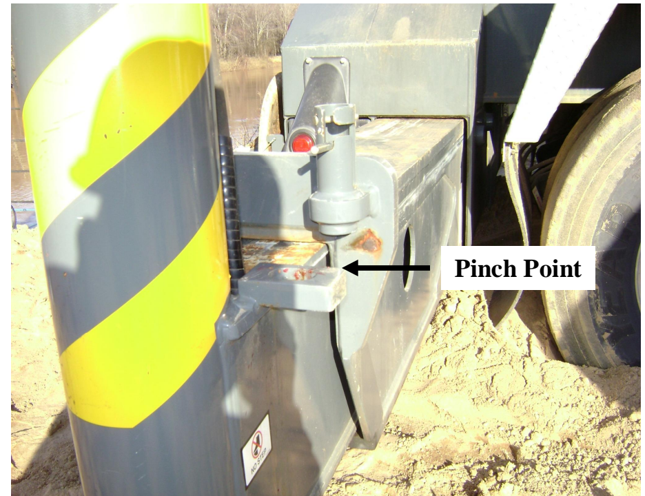
Telescoping outrigger where miner was injured
