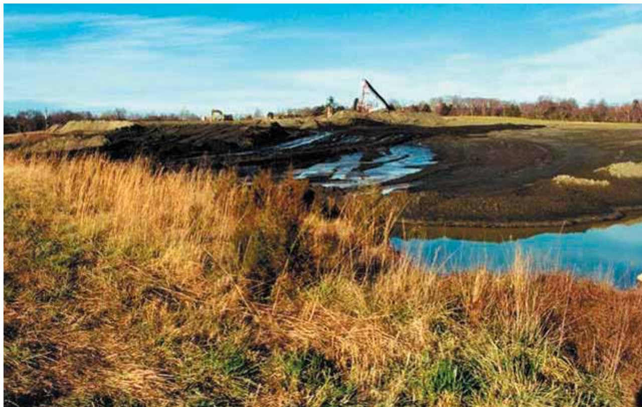
Figure 30. Open cut in weathered mafic rocks of the Green Springs pluton; Virginia Vermiculite LLC, Louisa County (photograph by Stanley S. Johnson).
