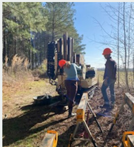
VA Energy geologists use a Geoprobe corer to collect Coastal Plain sediments, which helps with mapping in eastern Virginia.
