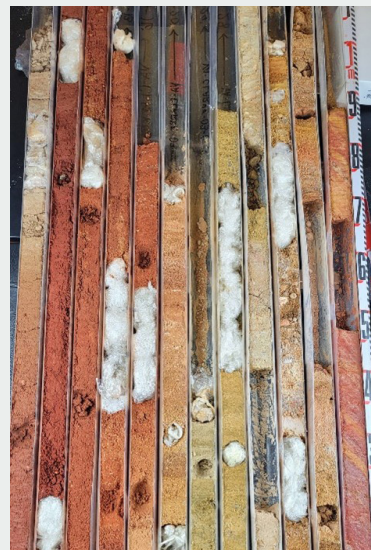
Coastal Plain deposits over foliated saprolite. Core was sampled for grain size analysis, geochemistry and geochronology in collaboration with the USGS.
