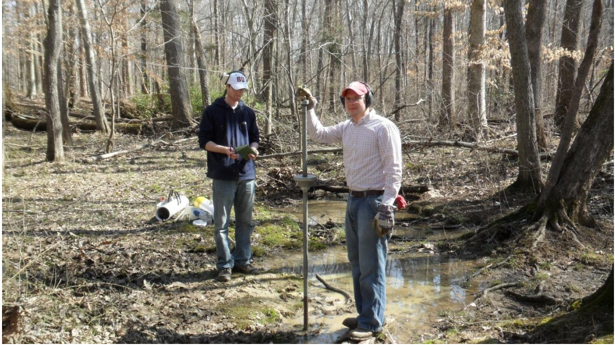
Figure 6. Sowers Dynamic Cone Penetrometer (DCP). Used to measure in-situ properties at the Yancey-3 and BOR-2 liquefaction sites.
