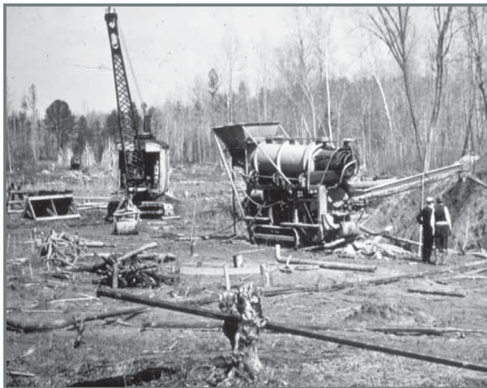
Dragline in operation in the early 1930s, Collins placer gold mine, Goochland County.
