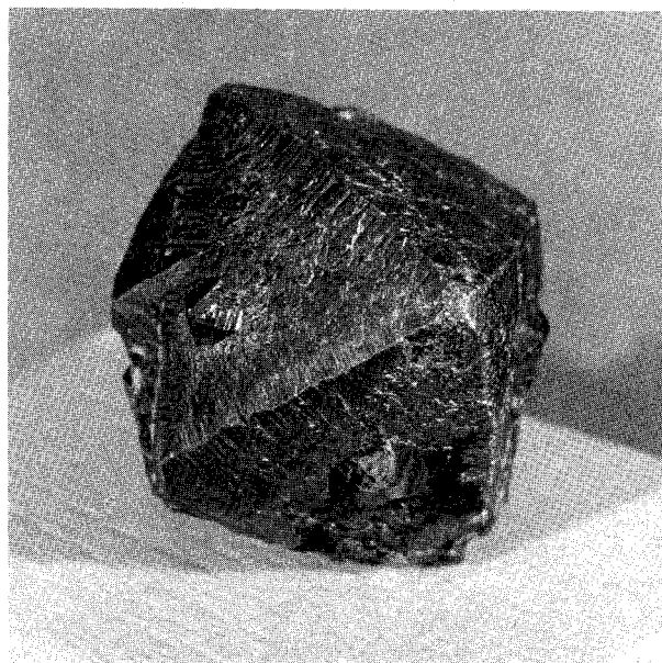
Figure 3. Intergrowths of large and small octahedral pyrite crystals; specimen 2 inches long (photograph by T. M. Gathright, II).
