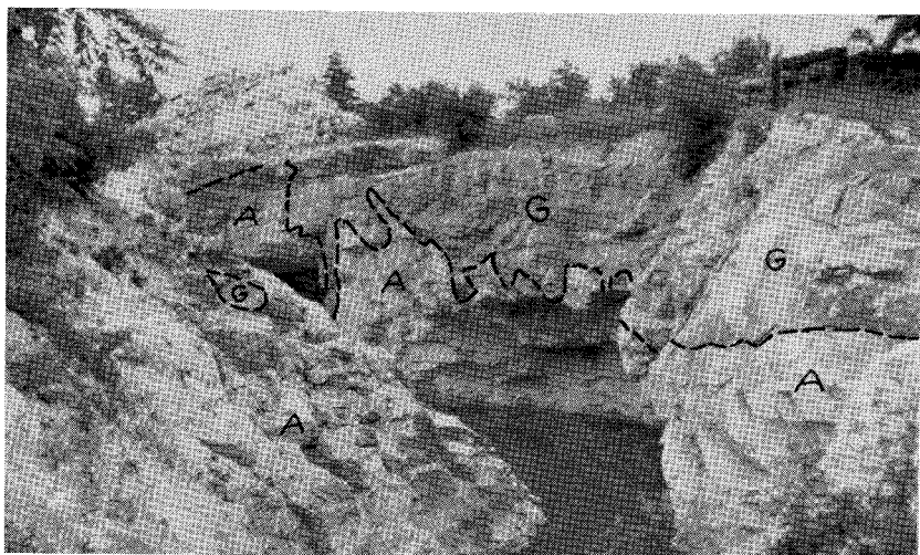
B. Peaksville alaskite-syenite mine, showing contact between light-colored alaskite-syenite, (A), and gray granite, (G).
