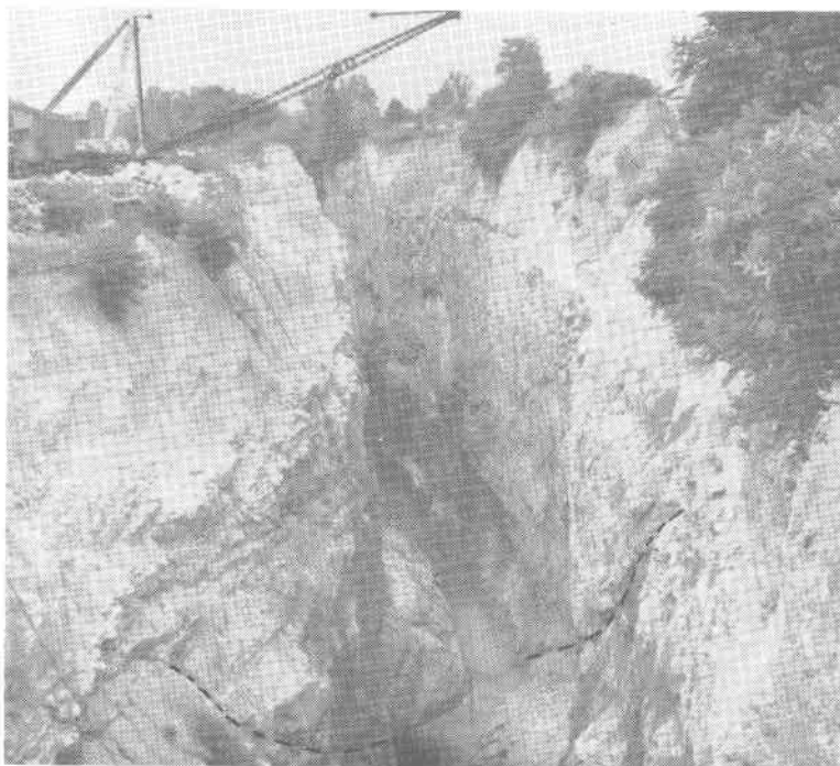
B. View looking southwest in the pit at the Patterson feldspar mine, Bedford County. The pegmatite is about 50 feet thick. Dashes show position of a minor fault cutting the pegmatite (1947).
