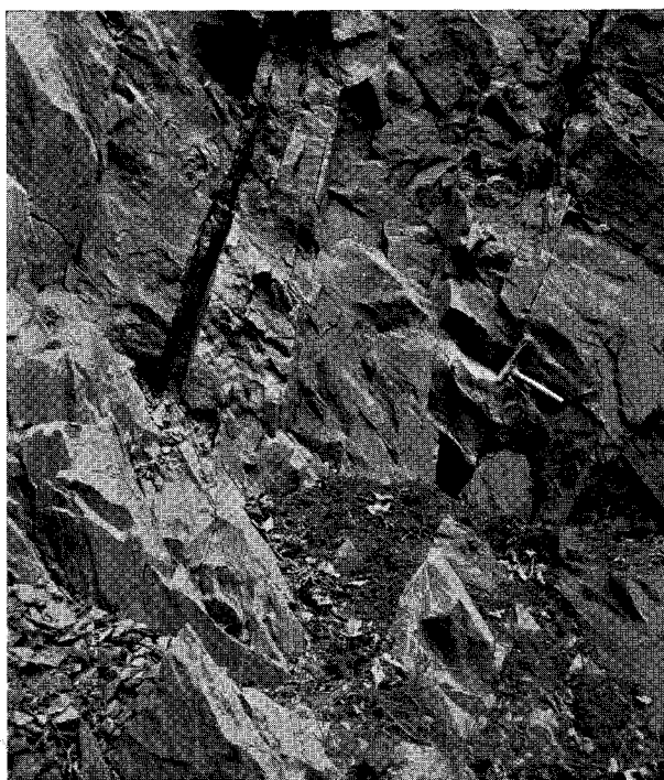
A. Quarry in massive Catoctin greenstone on the Lee Highway west of Warrenton. Note the scarcity of joints, which have been opened by blasting. One joint direction is shown.
