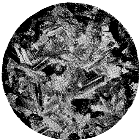
A. Photomicrograph of Triassic diabase sill in the southeastern corner of the Warrenton quadrangle, showing augite and labradorite. Crossed nicols. X 13.
