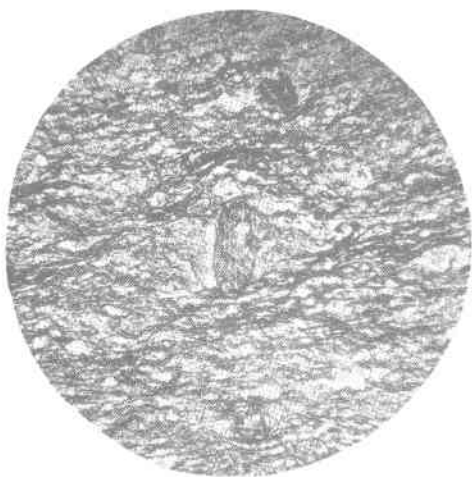
A. Photomicrograph of black slate of the Fauquier formation, about half a mile east of the bridge on the Lee Highway over Rappahannock River. The dark material is mostly graphite; the light material, quartz and feldspar. Plane polarized light. X 13.
