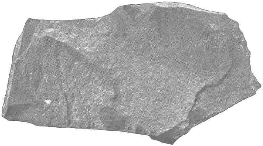
Fig. 2.—Fragment of highly argillaceous limestone or calcareous shale. Topmost layer of Chambersburg formation at Strasburg, Va.
