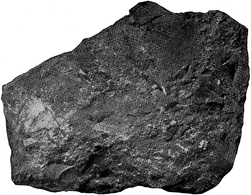
Fig. 1.—A mottled blue limestone, the darker, smooth areas being highly argillaceous and fine-grained, while the lighter speckled matrix is of much purer composition, and consists largely of crystalline calcite. Middle portion of bed 3a, Strasburg section, Strasburg, Va.
