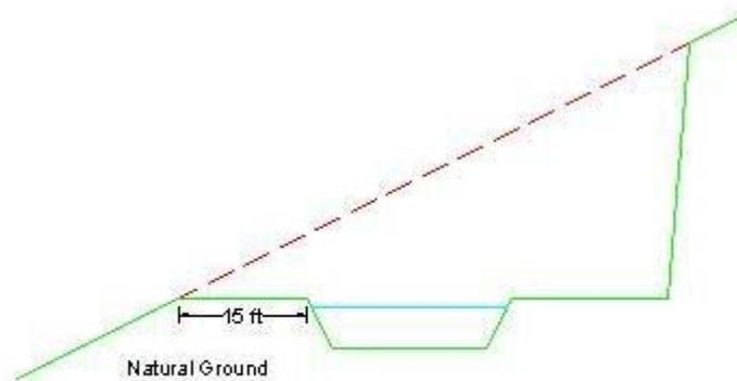
If the width between the top of the pond and the outslope is less than 15 feet then the pond will be treated as an embankment pond.
