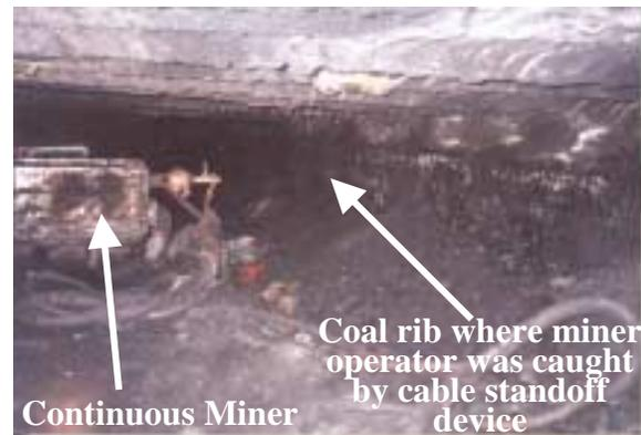
Machinery accidents continue to cause serious injuries and fatalities in the coal mining industry. Every person working in or around a coal mine must always stay alert to potential accident hazards when working around machinery. A continuous miner operator with only limited remote control miner operation experience at this mine received fatal injuries when he was pinned between the continuous miner cable standoff device and the coal rib. (photo's above)
